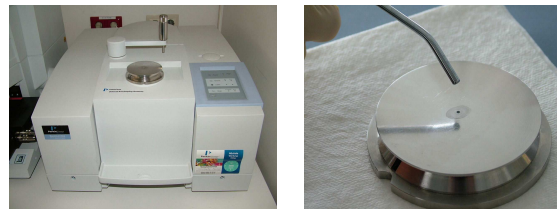
Figure 3: FTIR-ATR spectroscope, Spectrum One, Universal ATR Sample Accessory, Perkin-Elmer (left photograph) and prepared adhesive film on sample holder before measurement (right photograph).
