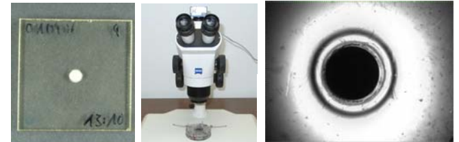
Figures 1 a/b/c: Preparation of the sample and measurement of shrinking force with polarized light.
