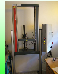
Photograph 7: Universal testing machine (Zwick Z010)
