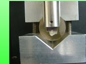
Photograph 6: Shear loading after 24h water storage at 37°C
