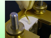
Photograph 3: Bulk filling of composite
