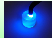
Photograph 2: Light activation of adhesive
