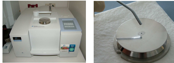
Figure 2: FTIR-ATR spectroscopy, Spectrum One, Universal ATR Sample Accessory, Perkin-Elmer (left photograph) and prepared adhesive film on sample holder before measurement (right photograph).
