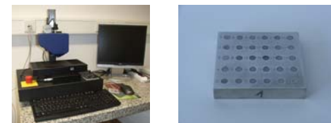
Figures 1 a/b: Surface laser scanner and metal mould for the specimen
